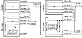
XIf the receiver OUT (black) line and the emitter JOB (black) line are not connected each other, the job indicator of the emitter is not operated and maintains the light status.
