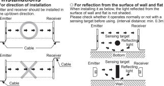
For protection of interference It may cause interference when installing more than 2 sets of the sensor. In order to avoid the interference of the sensor, please install as following figures and use the interference protection function
