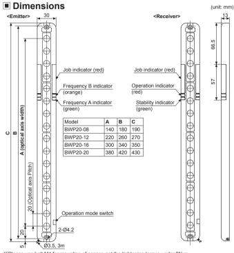
※Please use bolt M4 for mounting of sensor, set the tightening torque under 2N⋅m.
