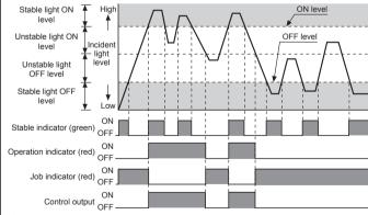
$\ensuremath{\mathbb{X}}$  The waveforms of operation indicator, job indicator, and control output are the state of operation for Light ON, but in case of Dark ON, it is opposite operation against Light ON mode
